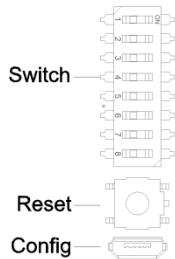
Switch: the DIP switch is used for setting the IP address (the default IP address is 192.168.1.200).
