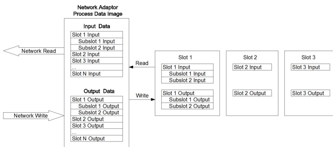
The maximum number of input bytes of the Ethernet/IP network adapter is 504 bytes, and the maximum number of output bytes is 504 bytes.
